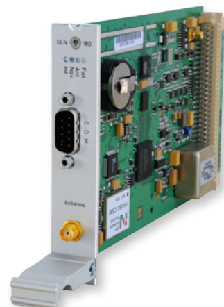
CLK Clock Module GPS, GLONASS, PZF
