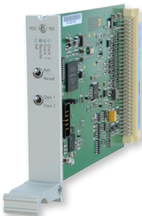
RSC Switch Card for seamless Signal Changeover
