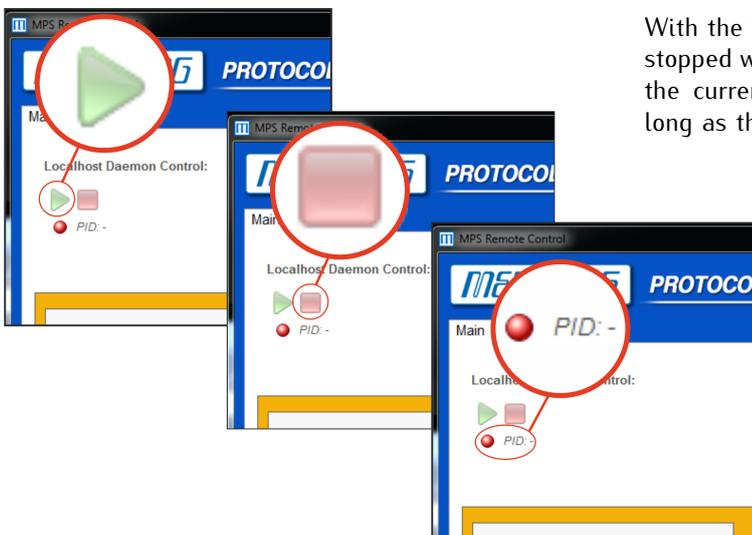
With the "Play" button, the service can be started and stopped with the "Stop" button. In the "PID" area, both, the current status and process-ID are displayed, as long as the service is running.
