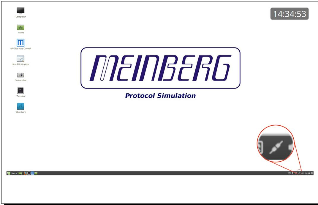
After logging-in, click on the marked symbol on the right side at the lower edge of the screen and after that on “Network Settings”. In this field you can make settings for the network adapter.
