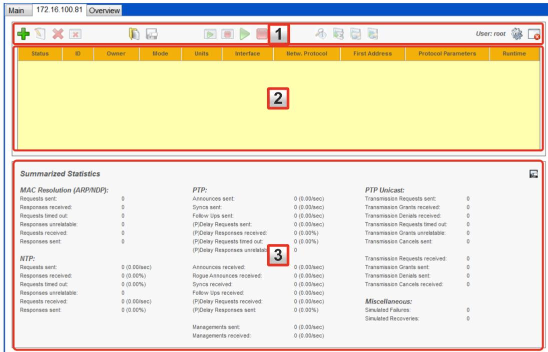
In area 1, the main menu to configure, control and monitor the simulation service, is displayed.
